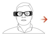
The goggle has been designed for quick and easy placement. At a mere 60 grams there is no slippage. Calibration is quick and easy, using two lasers that are incorporated into the goggle itself, eliminating the need for any additional hardware.
